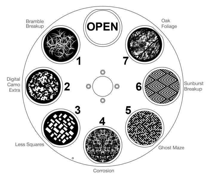
Figure 1-1: Fixed Gobo Wheel Illustration
