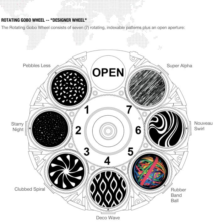
Figure 1-2: Rotating Gobo Wheel Illustration
