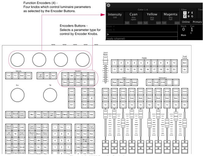
Figure 1-2: V276 Encoder Controls
