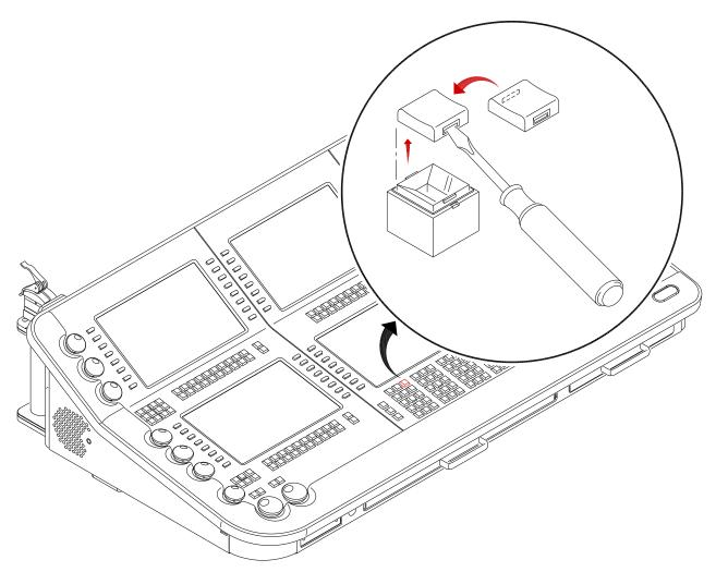
Figure 3: Replacing a Key Cap
